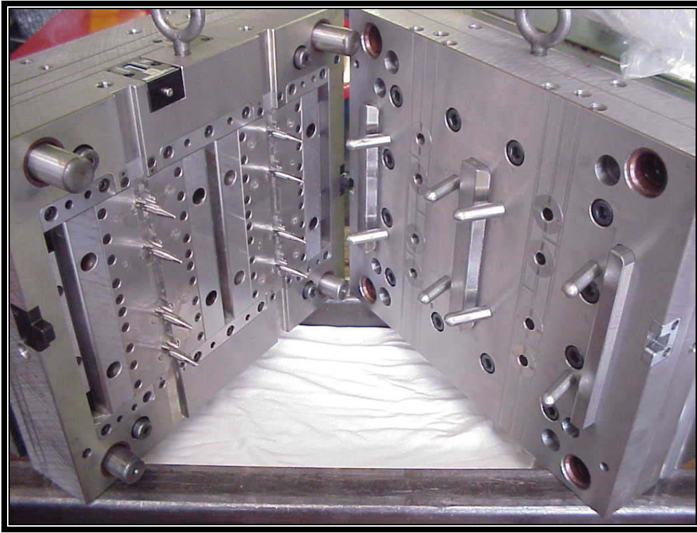
Figure 9 Cam action mold used in industry.
