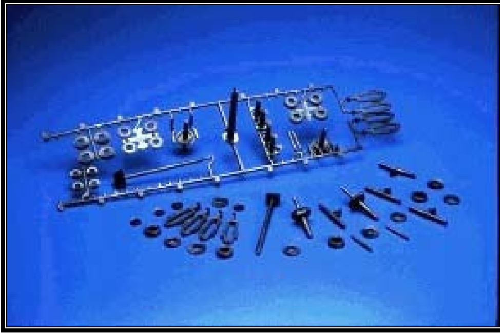
Figure 8 Modular molding trees with many parts
