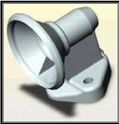
Figure 10 Injection molded part requiring cam action
