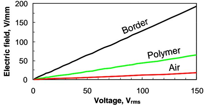
Fig. 2. Electric field within the LC layer at the lens border and lens center with various voltages applied across the electrodes. The LC cell gap is 25  $\mu\text{m}$  and the sag of the glass shell is 0.72 mm. The filled material is either polymer NOA81 or air.
