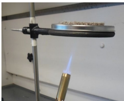
Figure 7: Indirect Heat Method burn setup
