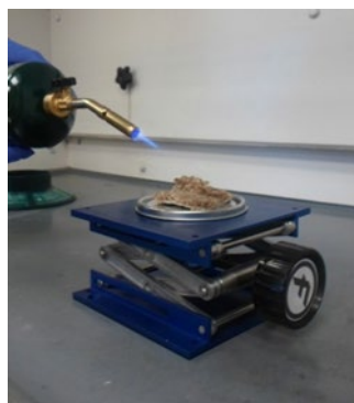
Figure 6: Direct Heat burn setup
