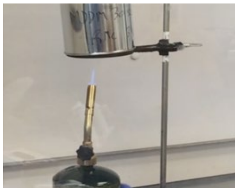
Figure 5: Modified Destructive Distillation Method burn setup
