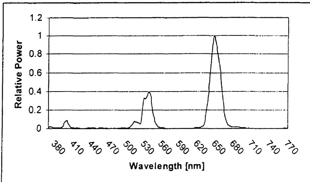
Figure 5. Emission from YF<sub>3</sub>:Yb,Er with continuous 980nm pump.
