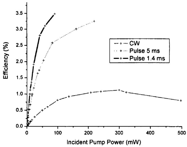
Figure 9: Efficiency of YLiF<sub>4</sub>:Yb,Tm for different pulse lengths
