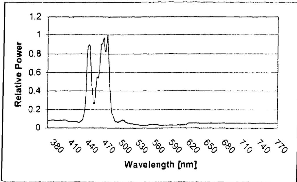
Figure 6. Emission from LiYF<sub>4</sub>: Th, Yb with continuous 980 pump.
