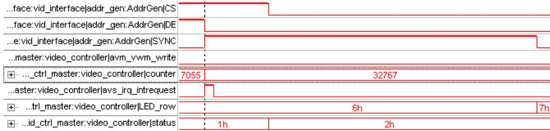
Figure 23: Video Controller Behavior at the End of a Sub-frame.
