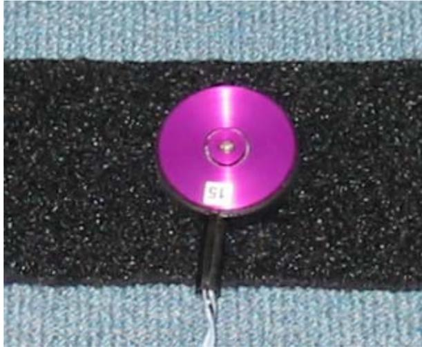
*Figure 5.* A Model C2 tactor secured to a Velstretch® belt
